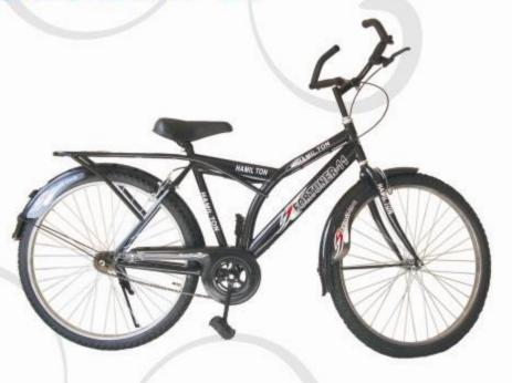
UNIQUE DESIGN FRAME WITH INBUILT STRONG CARRIER HEAVY DUTY FAT FORK HEAVY STEEL CHAIN COVER & MUDGUARDS. LO-RISE HANDLE BAR WITH STEM & GRIPS. BAR END, CALIPER BRAKE SYSTEM. MTB SADDLE, REFLECTORS FOR FRAME & CARRIER, REFLECTIVE PEDALS. SIDE STAND &
