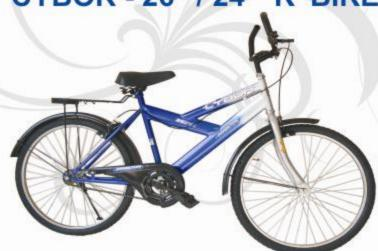
SPECIALLY DESIGNED K' FRAME WITH HEAVY DUTY FAT FORK. STEEL CHAIN COVER & MUDGUARDS. LO-RISE HANDLE BAR WITH STEM & GRIPS. BAR END, CALIPER BRAKE SYSTEM. CARRIER REFLECTORS FOR FRAME & CARRIER, REFLECTIVE PEDALS. SIDE STAND & STEEL RIMS.
